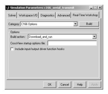
Observe that the **Build action** is Download\_and\_run. When you generate code for this model, it will automatically start a download utility program and load the application onto C166® microcontroller hardware over a serial connection. The code will then begin execution on the target.
