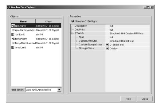
Here you can see the SimulinkC166. Signal data object and you can click on each object to inspect the properties.
