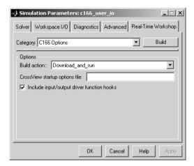
This instructs Real-Time Workshop to include extra calls to the user-supplied I/O device driver functions when code is generated for this model.
