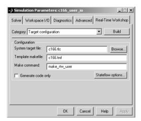
This command instructs Real-Time Workshop to compile and link the hand-coded I/O driver source files specified in the make file in the build process.
