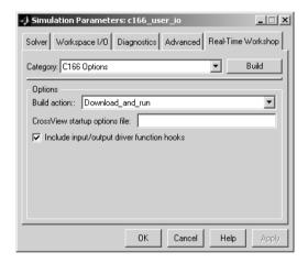
**3** Select the check box option for including I/O driver function hooks.
