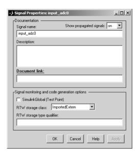
Observe that the **RTW** storage class is ImportedExtern. When you generate code for this model, Real-Time Workshop will use the specified variable name input\_adc0 and will create an extern declaration in the model header file. Since the Real-Time Workshop storage class is ImportedExtern, this variable must be defined in the hand-written driver code. When you open the file user\_io.c in the next step, you will find the line uint16\_T input\_adc0 that provides this definition.
