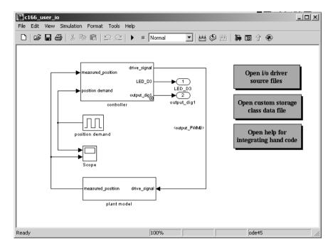
2 Open the controller subsystem by double-clicking and select the signal input\_adc0<>.
